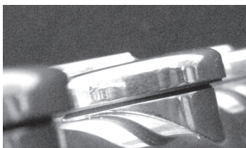
Soft soldered tone holes, not drawn and rolled.
